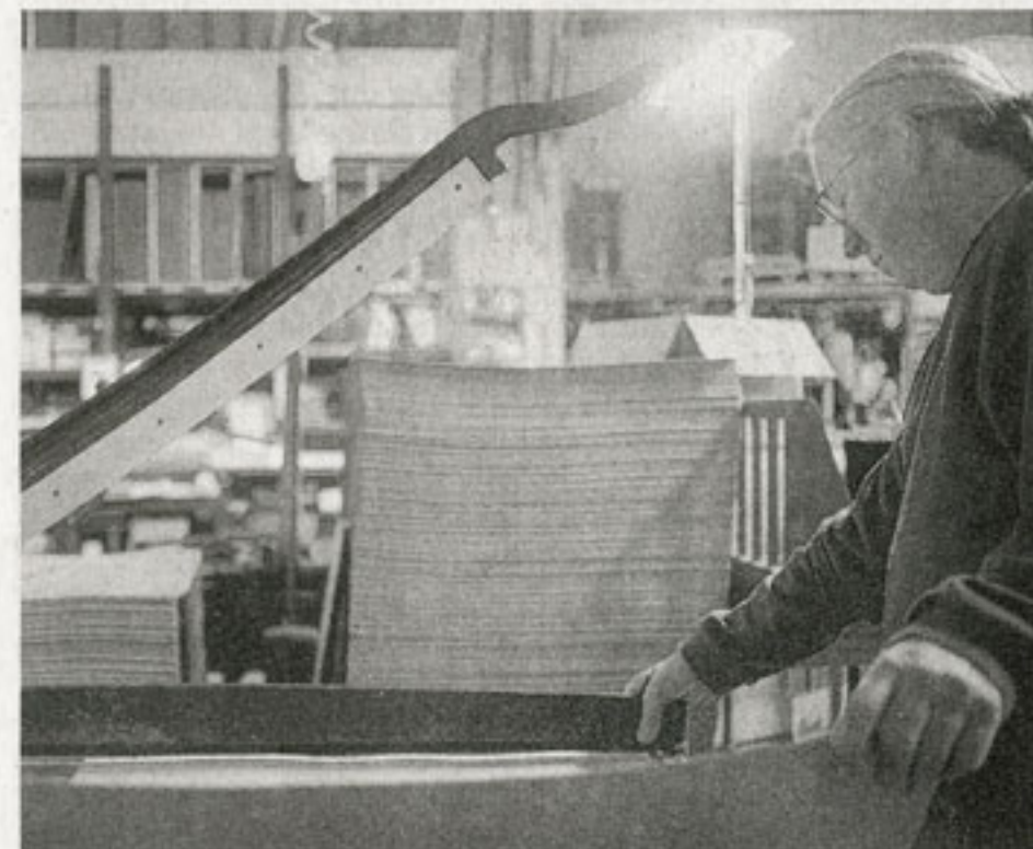
To create a book cover, book board is cut into pieces, before being covered by book cloth.
